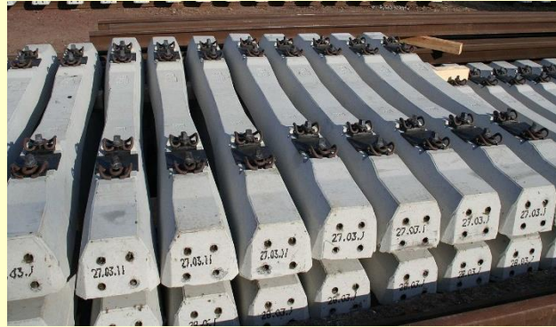
Single block reinforced concrete
