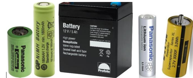
From left to right : NiCd, NiMH, lead-acid, Li-Ion, Supercapacitor
