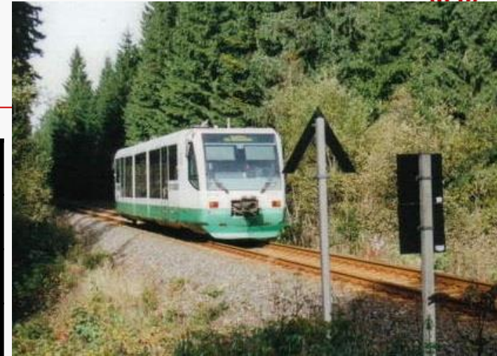
Siemens DUEWAG Regio Sprinter DMU on Vogtlandbahn railway tracks
