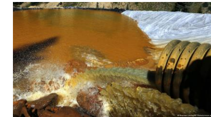
Yellow-brown acid mine drainage flows into a wastewater pond in efforts to reduce heavy metal and chemical contaminants
